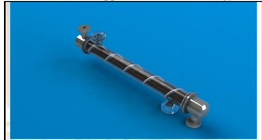
Figure 3 Shell and Tube heat exchanger with continuous helical baffle
